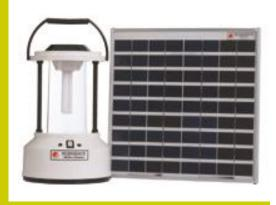
Solar lantern is an omni directional and portable light source which emits pure white light. It consists of sealed maintenance free lead acid battery (SMF), solar module, charge controller and DC-AC inverter for lighting the compact fluorescent lamp (CFL).
